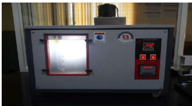
Figure 3: Cannon-Fenske Viscometer with oil sample
