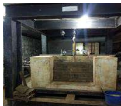
Fig. 1 Test tank and loading frame
