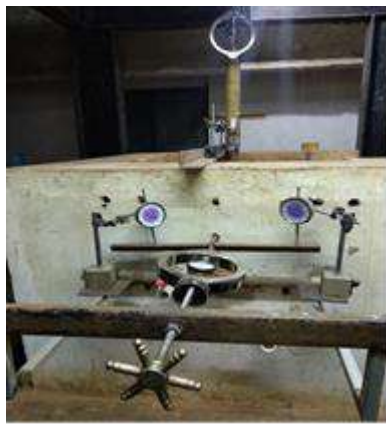
Fig. 3 Arrangement for Lateral loading
