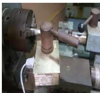
Figure 9: Lathe setup with tool dynamometer
