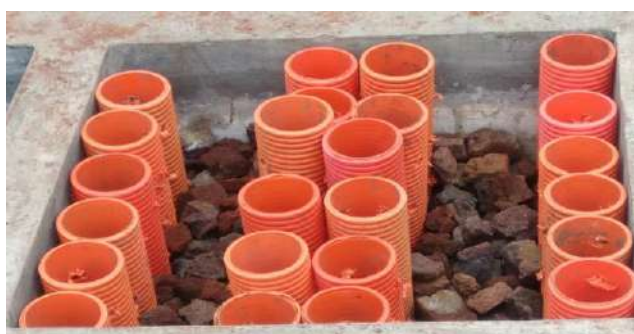
Fig.1 Photographic view of Bio-rack pipe without vegetation
