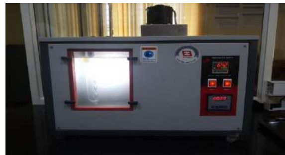
Figure 2: Cannon-Fenske Viscometer with oil sample
