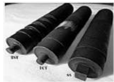
Fig.8. square, threaded cylindrical and threaded square tool [27]
