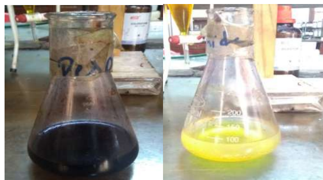
Figure 6: Change of colour of oil sample before (left) and after (right) titration for peroxide test.
