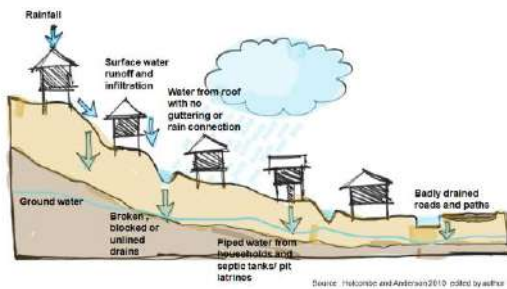
Fig. 7. Surface water flow modifications due to unauthorized constructions over hill area (Source-Author)
