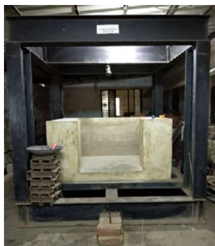
Fig. 1 Test tank and loading frame
